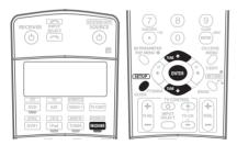
**1** While pressing the RECEIVER button, press SETUP. The remote LCD display shows SETUP.
